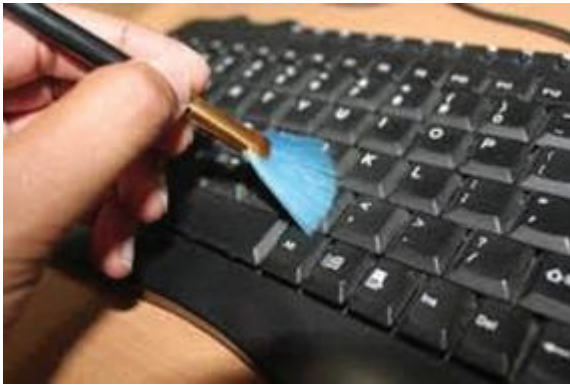
Figure 3.21: Cleaning keyboard with soft brush
